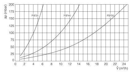
Pressure drop versus throughput (water, 20 °C)
